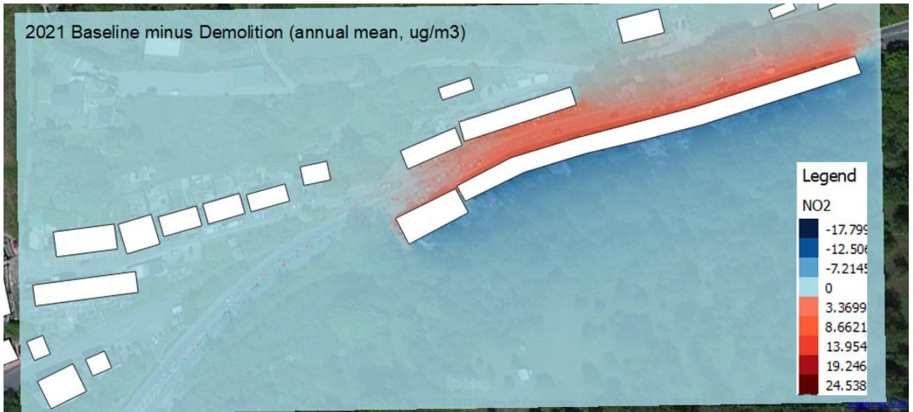
Figure 4-12 NO 2 difference plot for 2021 Scenario 3 (red areas = lower NO 2 concentrations, blue = higher)
