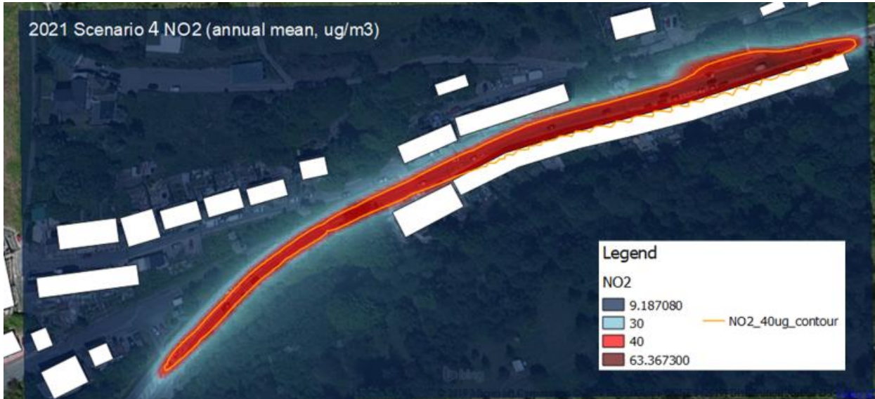
Figure 4-15 NO 2 exceedance / compliance plot for 2021 Scenario 4 (green dots ≤ 40 µg/m 3 , red dots > 40 µg/m 3 )
